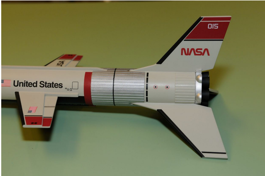
Photo 16: Finished Corrugated Wrap, with Booster Joint
