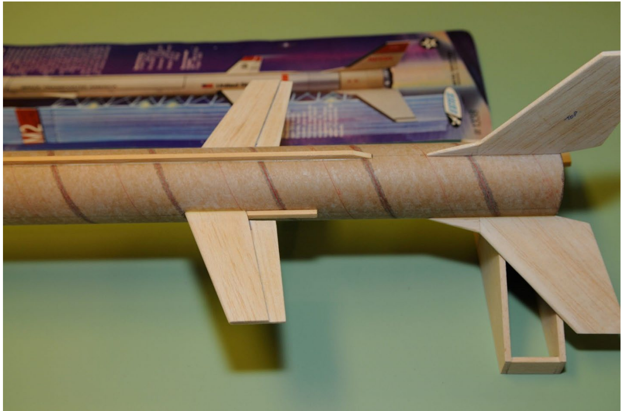
Photo 6: Dorsal Strip Stock Installed
